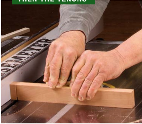
Shoulders and ends. Define the shoulders with the miter gauge (left). Now you can load the workpiece in your tenoning jig and make the cuts that will form the ends of these twin tenons (right), checking the fit by inserting the workpiece partway into one of the mortises.
