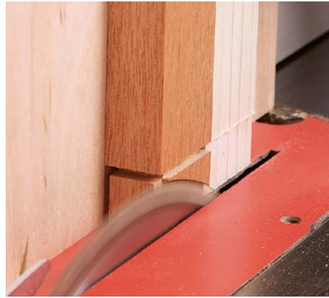
Shoulders and ends. Define the shoulders with the miter gauge (left). Now you can load the workpiece in your tenoning jig and make the cuts that will form the ends of these twin tenons (right), checking the fit by inserting the workpiece partway into one of the mortises.
