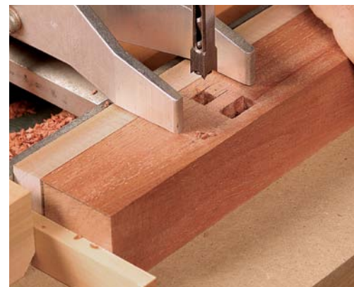
Add a second spacer and repeat. This spacer sets the distance between the mortises and is cut long to fully support the workpiece. Note that if the mortises are not precisely centered on the leg, you'll have to reverse the setup for the opposite leg.
