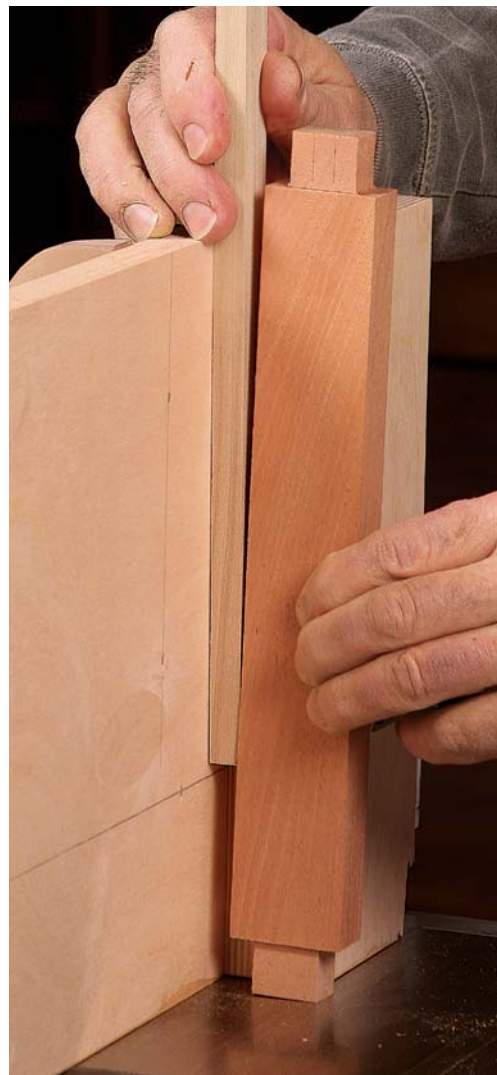
Spacer block sets up the inside cuts. The blade will next cut the inside cheeks, so the spacer should be the width of the tenon plus the blade kerf width (left). As with the tenon cheeks, you just flip the workpiece to make the second cut (right).
