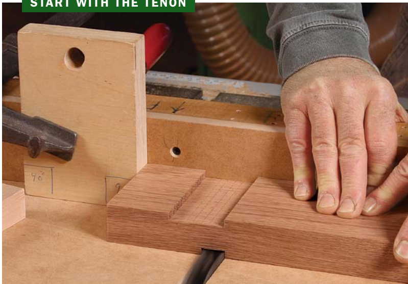
Stop block for one side. Cutting against the stop block defines the first wall of the two opposite dados.
