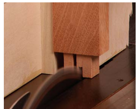
Spacer block sets up the inside cuts. The blade will next cut the inside cheeks, so the spacer should be the width of the tenon plus the blade kerf width (left). As with the tenon cheeks, you just flip the workpiece to make the second cut (right).
